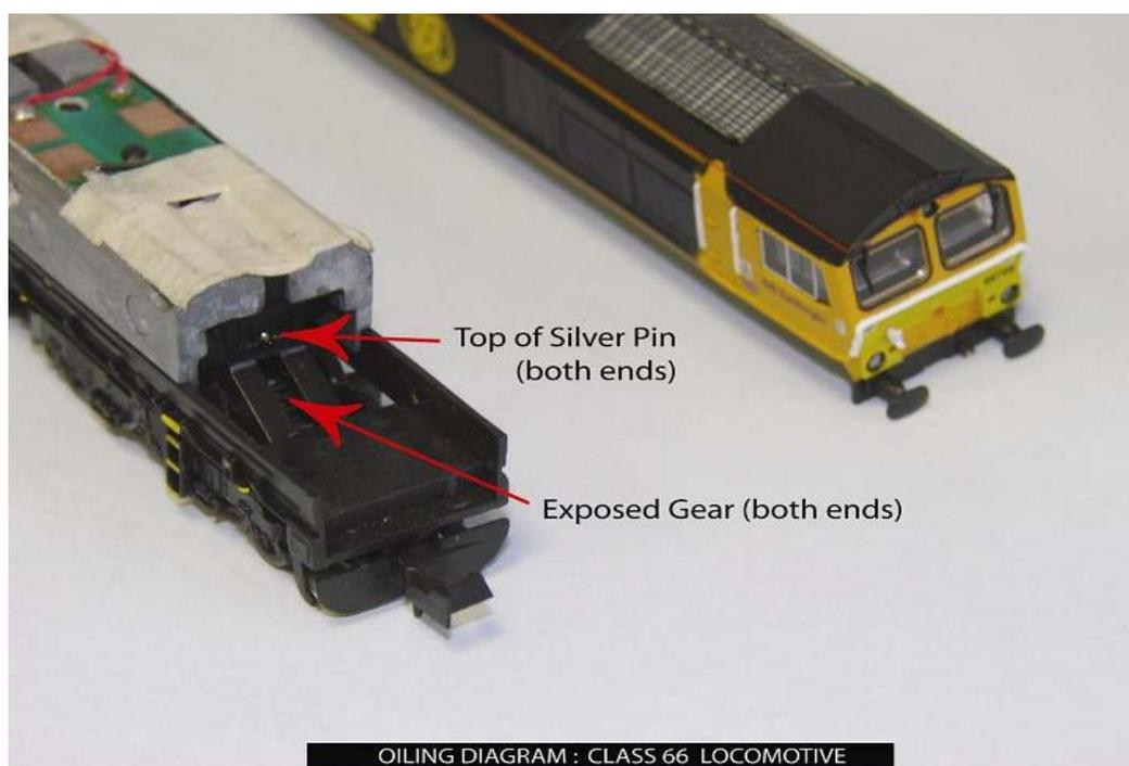
Experience has shown that since the original oiling instructions were issued with each model, these further 2 oiling points have been noted to radically improve running by thoroughly dissolving any 'transit' grease that may have been left in the upper part of the mechanism hindering running.
